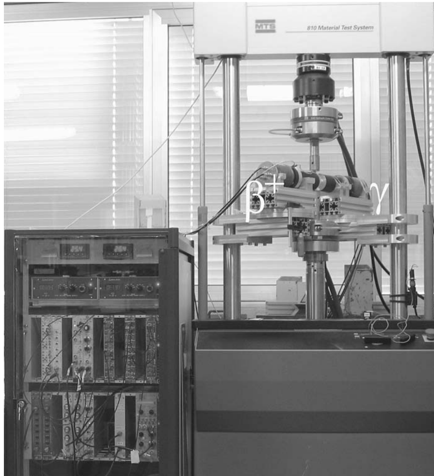
Figure 2 Integration of the \beta^+ and \gamma detectors in the load train of a servohydraulic testing machine. The photo multiplier tubes are magnetically shielded in a mumetal cylinder. The positron generator is integrated in the tip of the light guide of the \beta^+ -detector. The 511 keV annihilation photons are detected in a \text{BaF}_2 scintillator on top of the second photo multiplier ( \gamma ) (see also Fig. 3). The nuclear electronics is housed in a temperature stabilized box left to the load frame.
